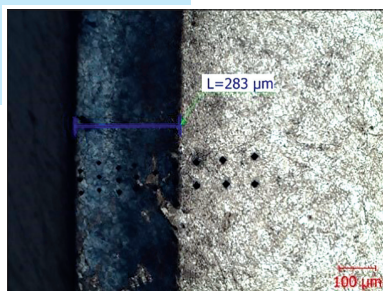
Fig. 3.39 Imprints of microhardness measurements (etched polished)
