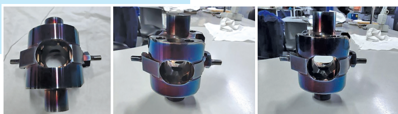
Fig. 4.3 Hydraulic units cradles with Avinit C310 nanocoating
