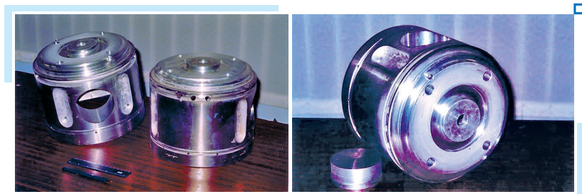
■ Fig. 3.58 Pistons D80.0406-1 of the D80 diesel engine with Avinit C220 anti-scoring wear-resistant coatings
