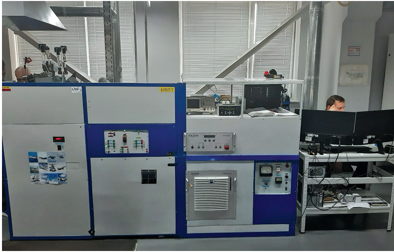
Fig. 2.4 Avinit V Unit (CVD)
