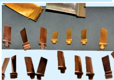
□ Fig. 3.29 Avinit C350 coating based on (Ti-Al-N)
