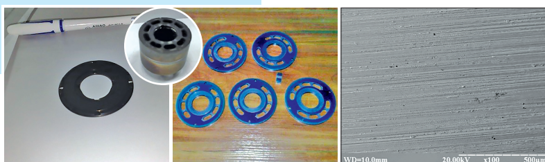
Fig. 3.57 Parts of aircraft units coated with molybdenum disulfide
