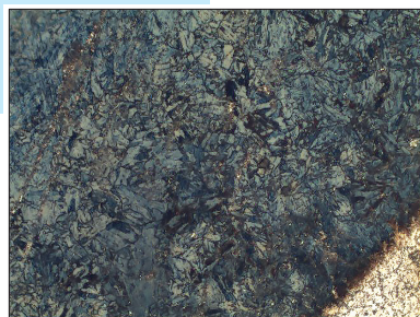
■ Fig. 3.36 The microstructure of the nitrided layer on 34NiCrMoV14-5 steel (×500)
