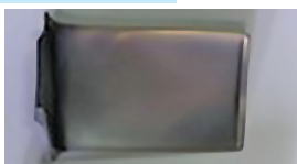
□ Fig. 3.30 Avinit D100 coating based on Ti-C
