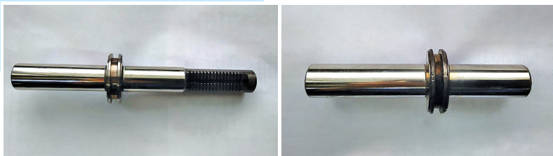
■ Fig. 3.32 Aviation units stems with molybdenum-carbide Mo-C coating
