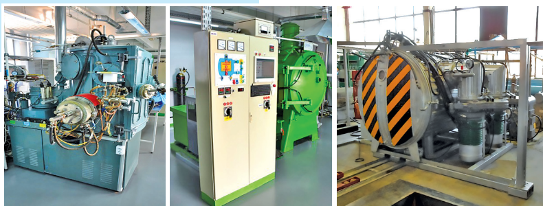
□ Fig. 2.1 Vacuum-plasma cluster Avinit
